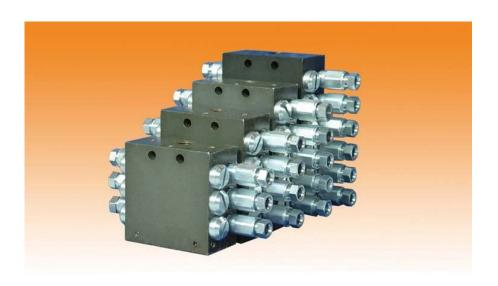
The SMP is a single block progressive divider valve that is ideal for applications where space is limited. It is available in 6,8,10 and 12 outlet versions, each with an output of 0.2 cm<sup>3</sup> / 0.012 cu. inch per cycle.
