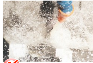
Machining with flood coolant
