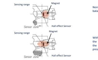
Normally, the magnetic field is balanced around the hall sensor.
