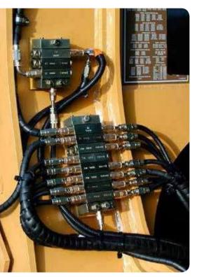
In progressive automatic lubrication systems, a piston pump supplies a deined amount of lubricant through the main line to the metering device that serves each outlet. SKF ProFlex and Lincoln Quicklub systems are designed for speciic applications and can be conigured to meet the unique lubrication requirements of every lubrication point on the equipment.
